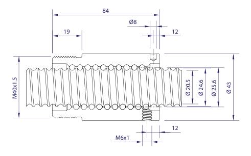
Ball bearing nominal diameter 5.0. Average ball quantity per nut is 68.
